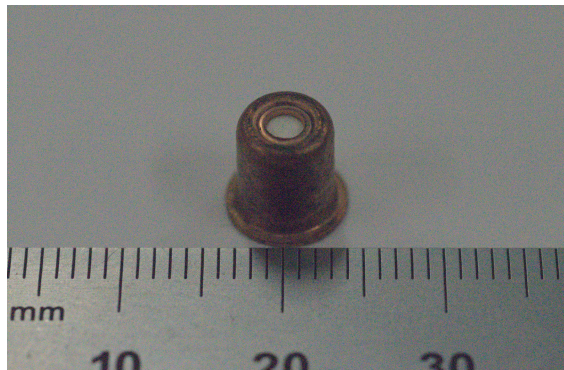
Figure 2.1: A Winchester 209 shotgun primer. The vent hole is the the white circular region on top of the primer.
