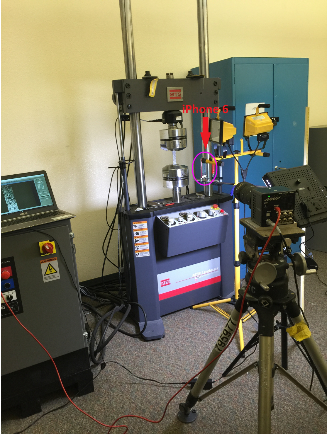
Figure 3.6: Experimental setup for iPhone test, using an aluminum speckle patterned sample. the multi-camera setup results in the iPhone set slightly off center-axis.
