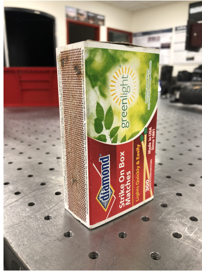
Figure 3.15: A box of matches was chosen as the object to reproject because of its known dimensions and unique features that can be used to correlate matching regions in the left and right camera.
